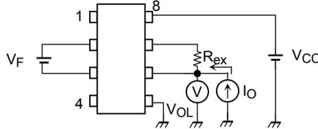
Test Circuit 2: IO2L
